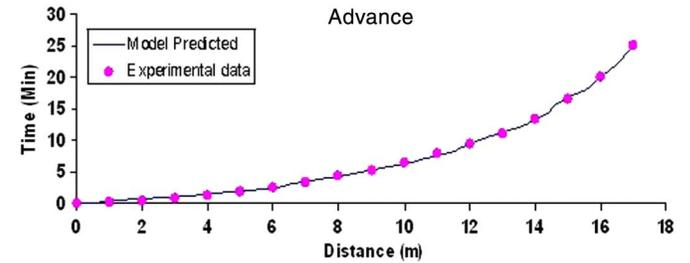
Fig. 5. Comparison of model-predicted and experimentally observed advance for border-strip 2
