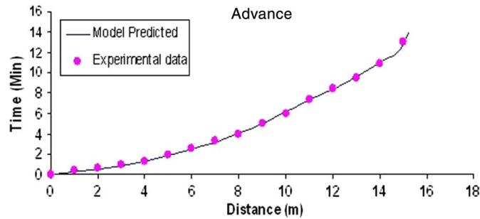
Fig. 2. Comparison of model-predicted and experimentally observed advance for border-strip 1
