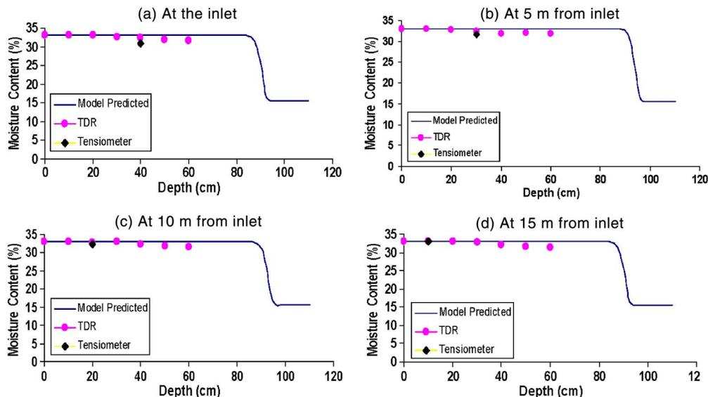
Fig. 4. Comparison of model-predicted and experimentally observed moisture content profile for border-strip 1 (at cutoff time)
