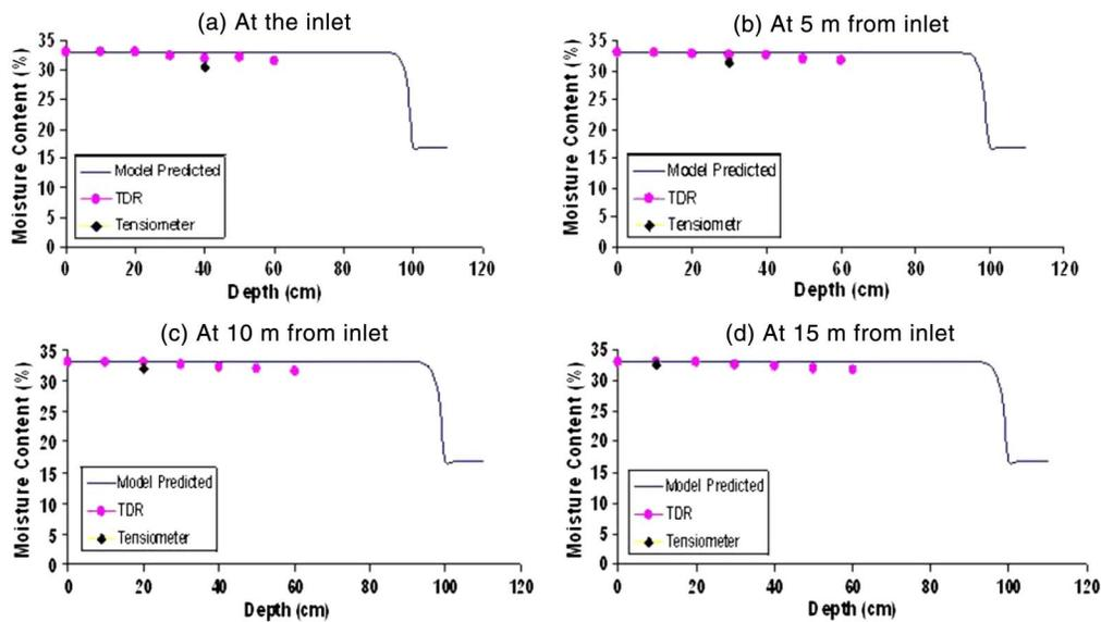
**Fig. 7.** Comparison of model-predicted and experimentally observed moisture content profile for border-strip 2 (at cutoff time)
