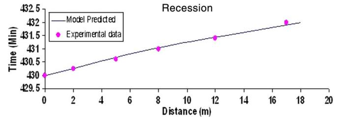
Fig. 6. Comparison of model-predicted and experimentally observed recession for border-strip 2
