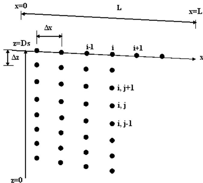
Fig. 1. Finite-difference numerical grid
