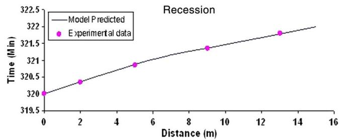
Fig. 3. Comparison of model-predicted and experimentally observed recession for border-strip 1
